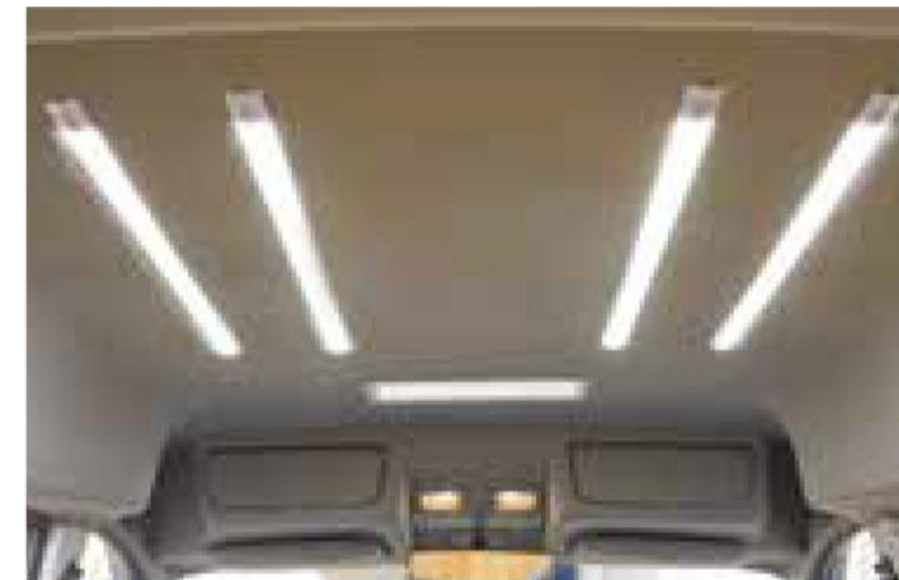
LED cargo lighting
